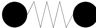
Fig. 3. One-dimensional test case involving two mass points linked by a spring with a stiffness and without structural damping.
